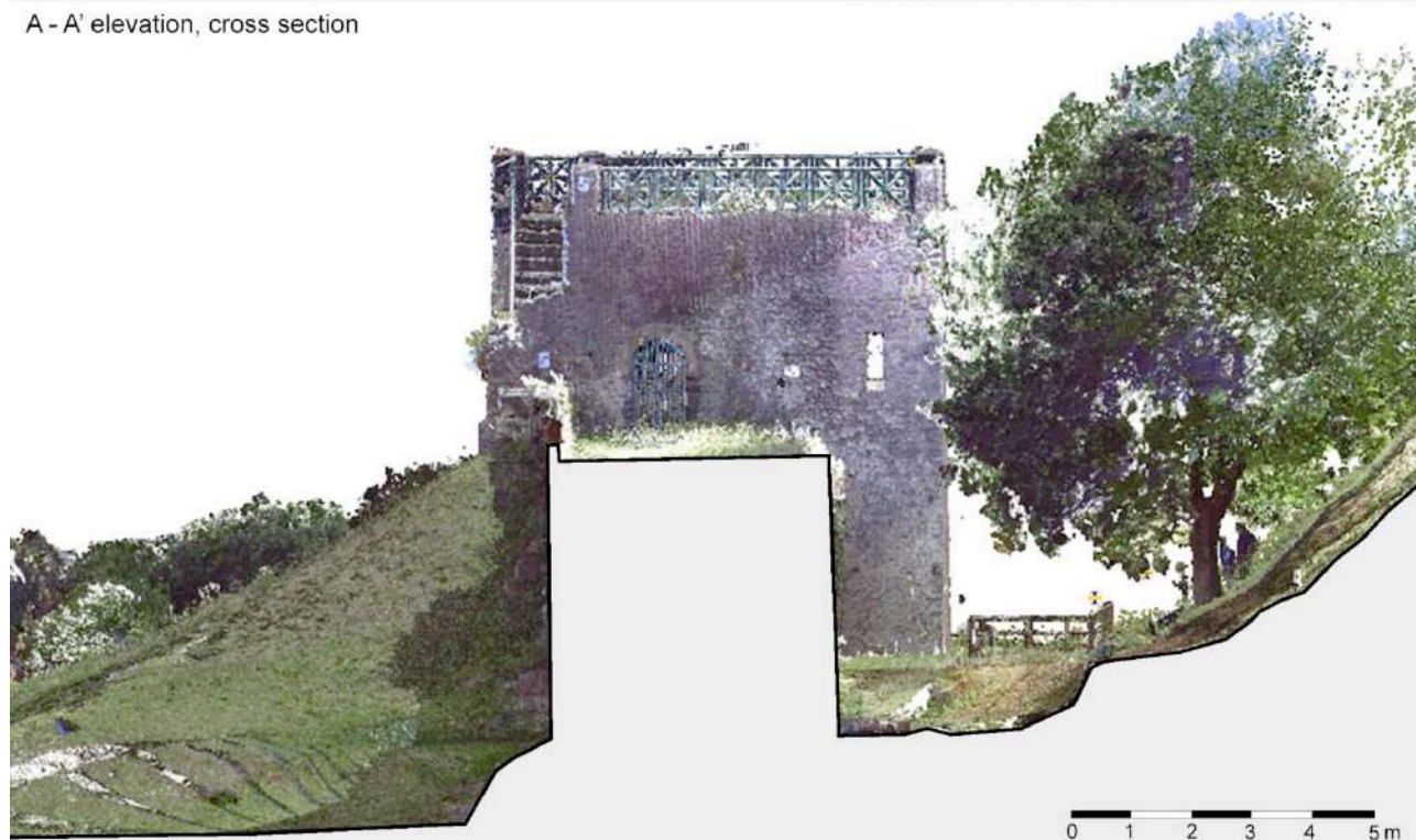
Fig. 6: Pompeii, Tower of Mercury. The 2d graphics of the tower were obtained through sections made on polygonal surface; redundant points were eliminated to check geometric inconsistencies that were in the mesh. The model has almost always gaps created by shadows. Four horizontal planes were drawn to realize plans at different altitude level. The sections had been useful to understand planimetric configuration of tower. The figure shows plan of 58 meter above sea level that is the ground floor. (Drawing by L. Abate, 2015).
