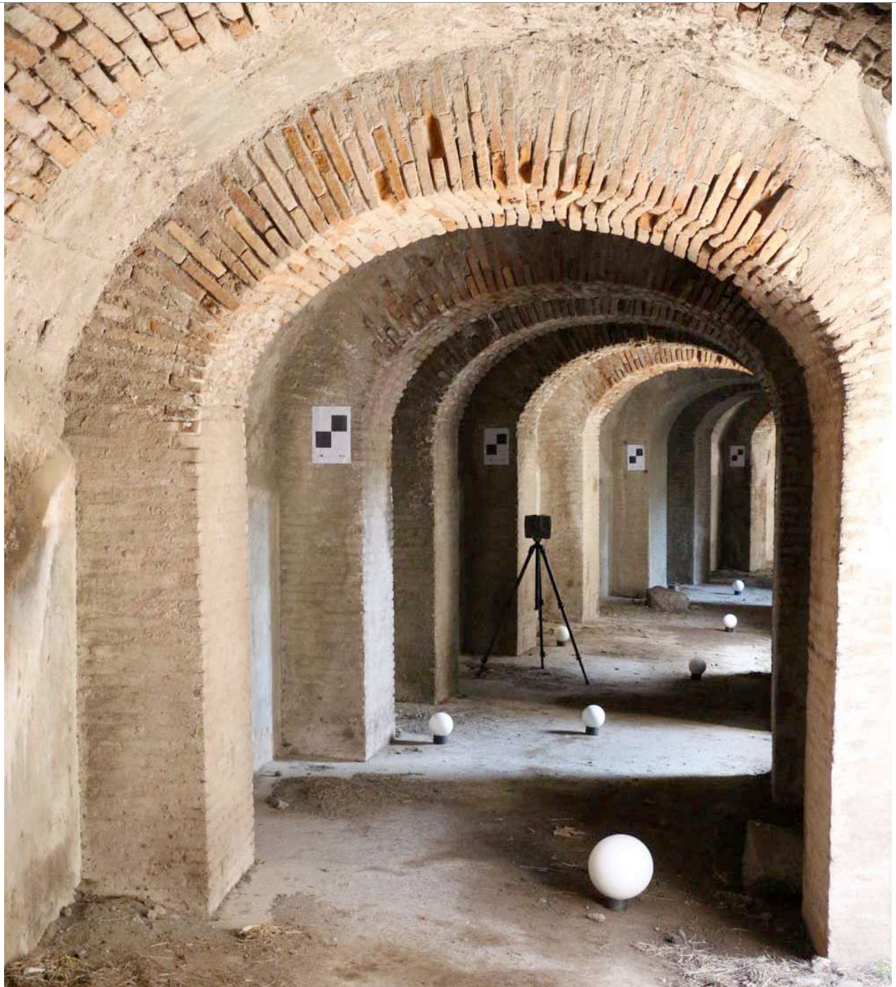
Fig. 35: Pompeii, Amphitheater. A instant view of the elliptical tunnel during the capturing laser data.
