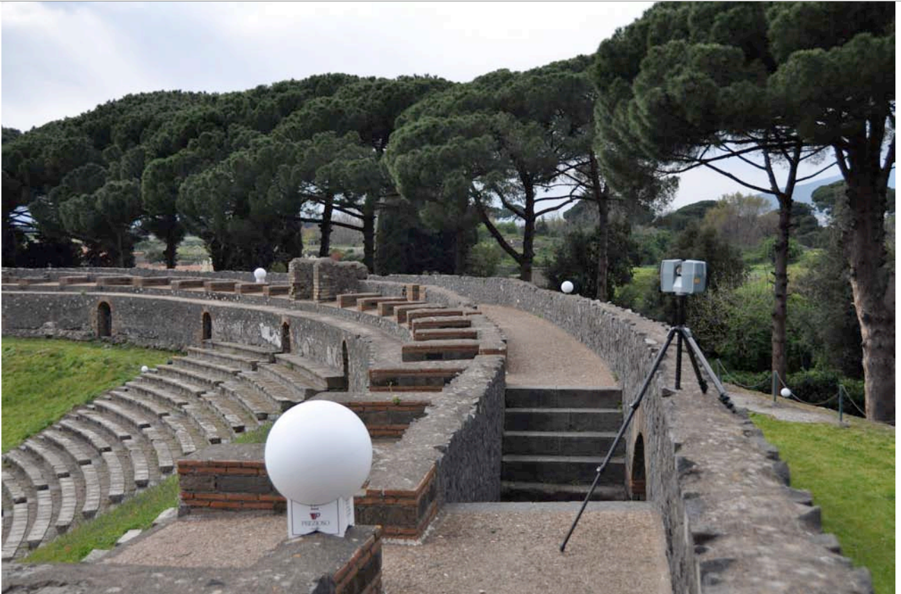
Fig. 27: Pompeii, Amphitheatre. A instant view of the upper walkway during the capturing laser data. In the scenario there are many white spherical targets.
