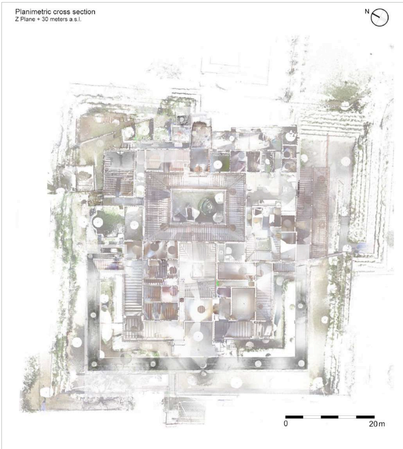
Fig. 15: Pompeii, Villa of the Mysteries. The figure shows the merge of 265 scans made for the survey of Villa of the Mysteries. The 2d graphics were obtained through sections made on polygonal surface (mesh); redundant points were eliminated to check geometric inconsistencies that were in the mesh. The model has almost always gaps created by shadows. In particular you can notice shadow cones represented by white circles in the figure, they are the position of the laser scanner in different phase of scanning. The figure is useful only for a visualization of Villa of the Mysteries, it is not a drawing accordance to UNI 936. (Drawing by R. Parente, 2015).
