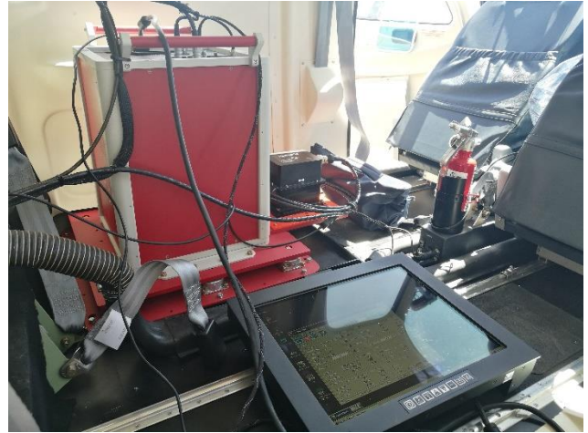
TABI-1800 TSR installed on Benecon's Aircraft
