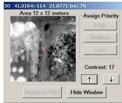
High resolution thermal thumbnails (brighter pixels=warmer temperatures, darker=cooler)
