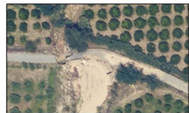
The acquisitions with the PhaseOne IXA camera allow to assess the damage to the infrastructure. The image shows the collapse of a road.
